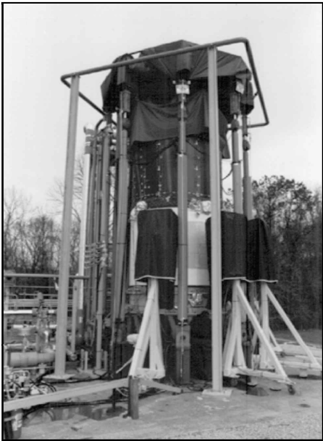
Fig. 26 MSFC structural testing of RLV liquid hydrogen tank.
