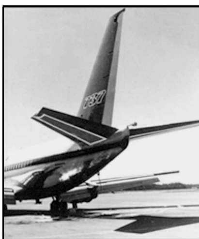
b) Boeing B-737 composite horizontal stabilizer
