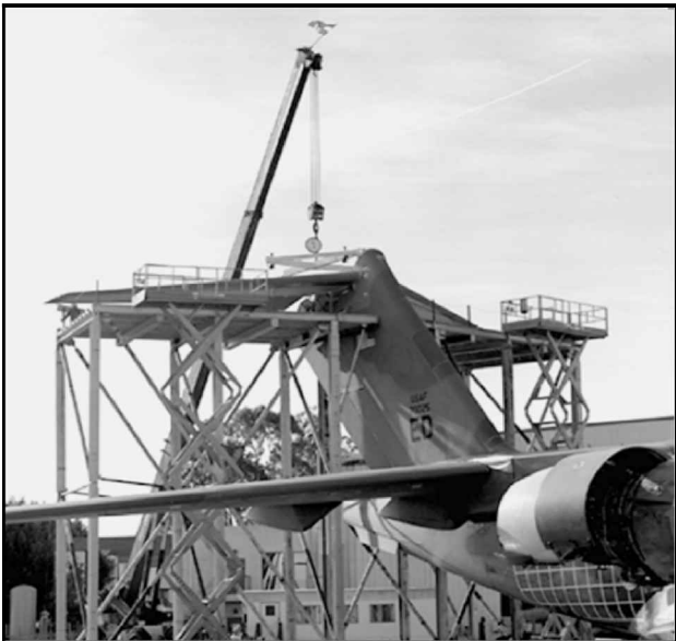
Fig. 10 C-17 horizontal tail redesigned using composite materials.
